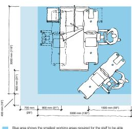
Blue area shows the smallest working areas required for the staff to be able to use the mechanical aids in an ergonomic way.
